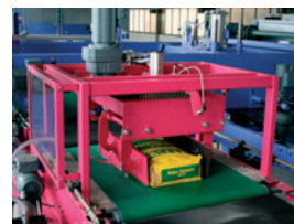
Flattening side flap rotator for soft bags
