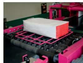
Lifting grate rotator for extremely limp bags
