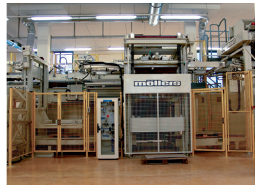
Corrosion-protected PLS-C palletizer in a packaging line for evaporated salt
