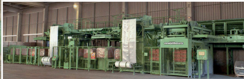
High capacity reverse hood shrinkwrapping packaging line
