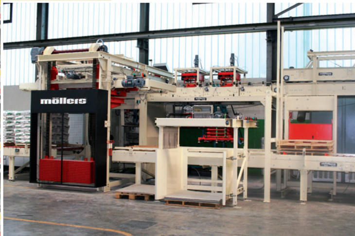
PLS palletizers in a dispatch terminal
