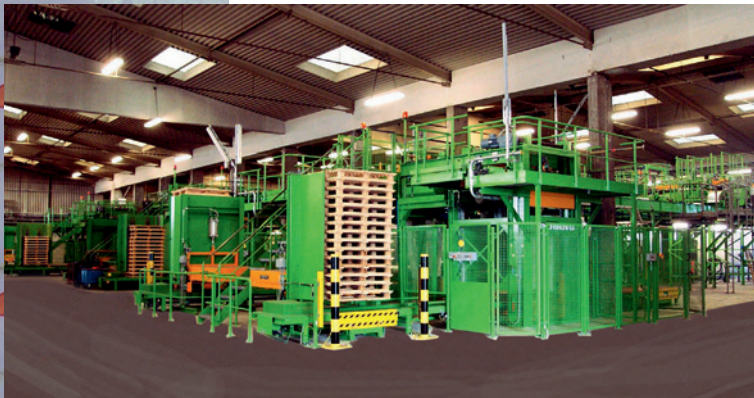
Large capacity packaging plant with six PLS-C palletizers in a polyolefin works
