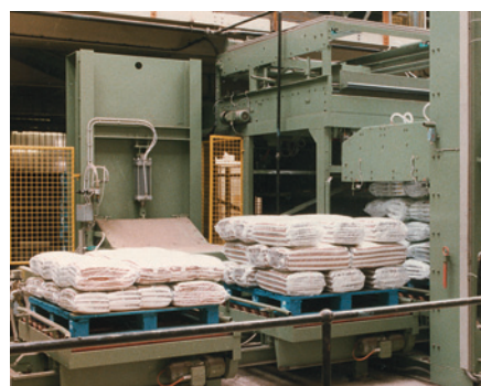
Multi-palletizers with three pallet positions
