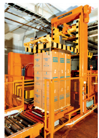
PFS special palletizer for large cartons
