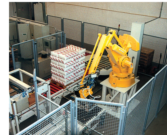
complete robot cell including empty pallet magazine, cover sheet placer and stretch wrapper
