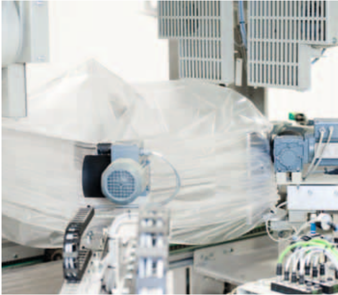
09. Hood Formation | Reefing of the size adjusted hood
