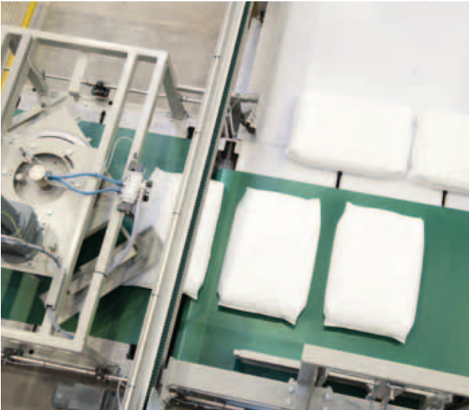
02. Gentle Bag Formation | Layers of packed goods are formed according to individual specifications
